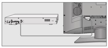
1 Connect the socket of the television and the corresponding socket of the video recorder, DVD player or set-top box with a SCART cable.
